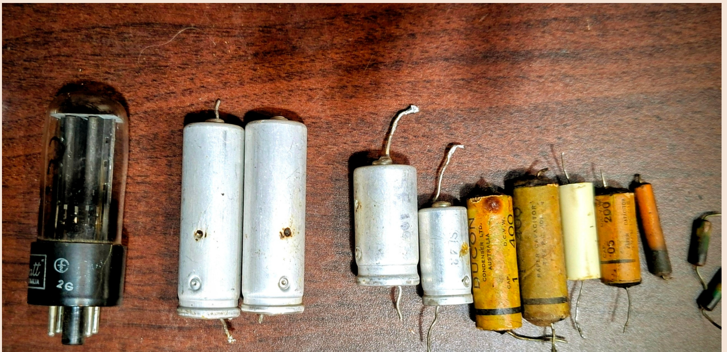
Fig 7 Parts after 77 years that had failed.
